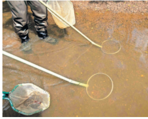
Electric "wands" send shock waves through the water, stunning fish and bringing them to the surface. Once the fish are identified, they are returned to the stream.
